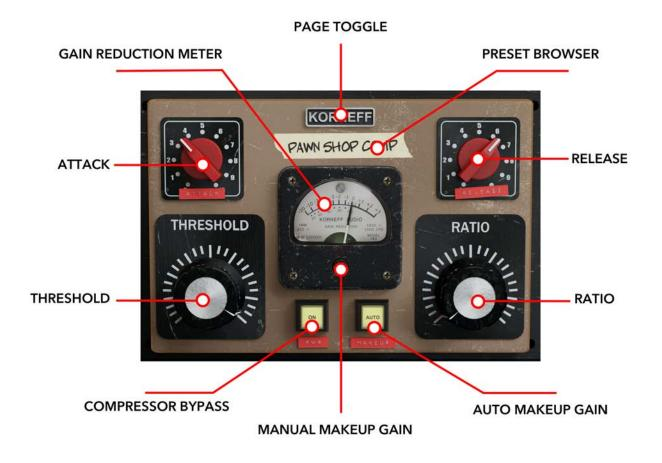
**ON** - press this to engage the compressor circuit. If you switch this off, the compressor is bypassed. Your signal will still go through the tube signal path, so you can still use the Pawn Shop Comp as a preamp and EQ.
