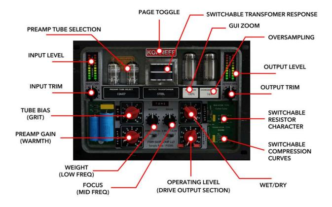
**PREAMP** - turn this clockwise to increase gain and add gentle saturation for more warmth and a slight lift in the high end (caused by added harmonic distortion).
